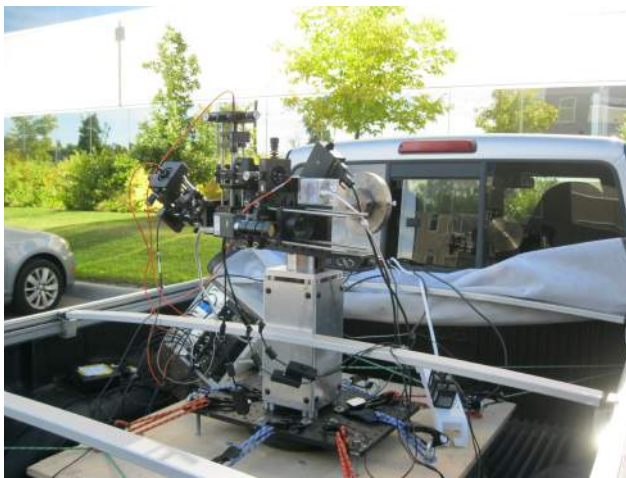
Figure 1: (left) Photo of the quantum key distribution receiver installed on the back of the pickup truck. The system is motorized with active velocity tracking using two-way beacon lasers. (right) QBER and photon count rate measured at the receiver during the measurement run. The horizontal gray line represents the mean signal QBER of the data selected for the QKD protocol (6.55%). The shaded regions around the QBERs correspond to a 95% central credible interval. The QBER drops when the count rate increases at 4-8 s. The large range of the credible interval of the decoy QBER is due to the low number of measured decoy states, with results near the beginning absent as no decoy states were measured at those times. The measured values are taken with a 0.16 ns coincidence window, with the QBER measured on a per second basis and the counts measured on a 2 ms basis.
